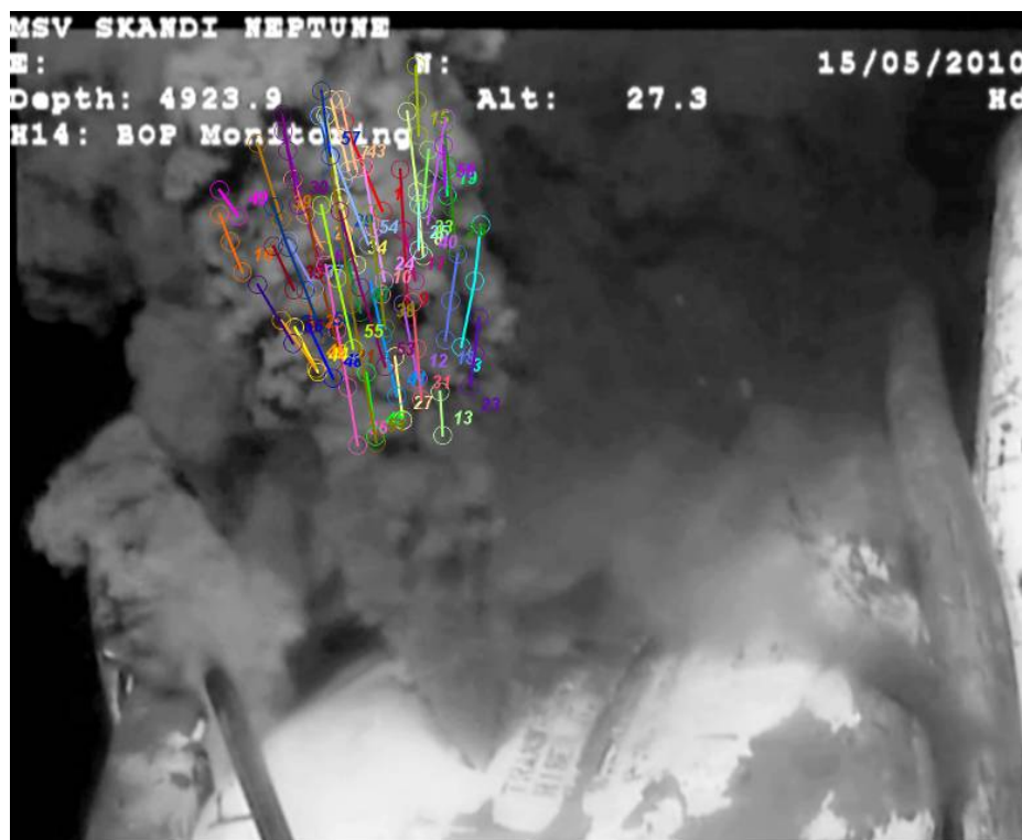
Figure 4: Manual feature tracing in the main jet of the Riser Kink Jets. (Trajectories were pseudocolored randomly to make them easier to see. The colors do not represent velocity magnitude).
