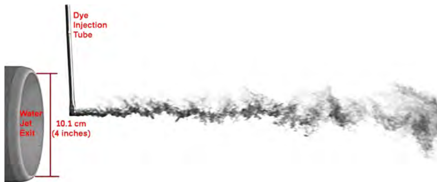
Fig. 4. Flow visualization with dye point injection. Water flow rate was 41.7 l/s (11 gal/s) producing a Reynolds number of 500,000. The camera frame rate was 1500/s and the exposure time was 0.75 ms.
