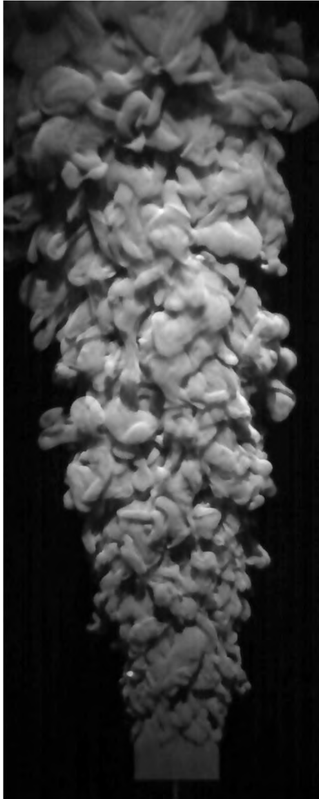
Figure 20. Water jet made visible with fluorescent dye. The intricacy of the jet-ambient fluid interface is clearly delineated. Q=1 gpm, Re=4500 .
