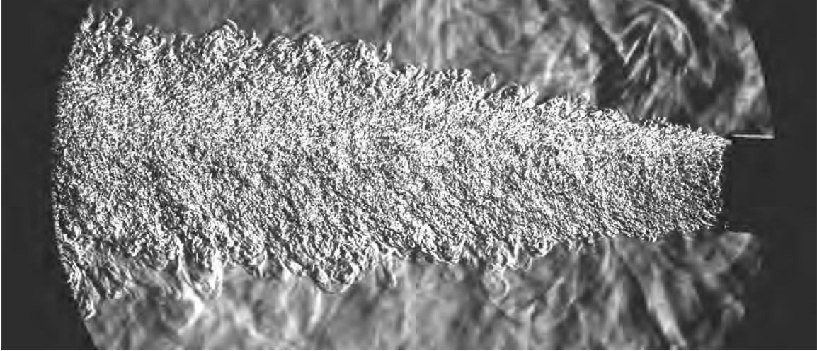
Figure 7. Schlieren photograph of water discharging vertically up into tank. The flow is made visible by slightly heating the discharge pipe exterior to the tank.
