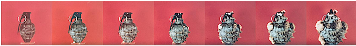
Electronic detonation of a hand grenade recorded at 2/3 million frames per second. Sequence taken by a Cordin Model 126 High Speed Rotating Mirror Camera. ©Cordin Co.
